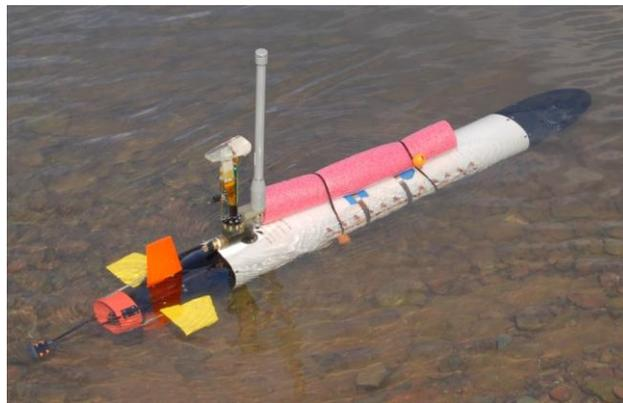
Fig. 1. Modified OceanServer IVER2 AUV
